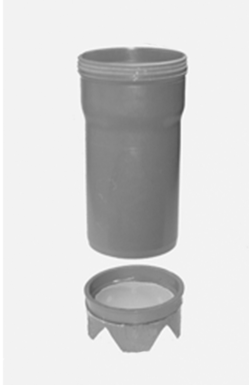
Figure. 1. The feather lice strainer is made of a 20 cm PVC waste pipe and a 6 cm high socket made from a pipe coupling, and equipped with a 400 micron plankton net. The internal diameter of the pipe is 10 cm. The pipe coupling has been cut so the wider part is 2 cm high, sawn through below and glued together with the plankton net in between. As the water must flow easily from the strainer the socket has been sawn so that it stands on four legs.
